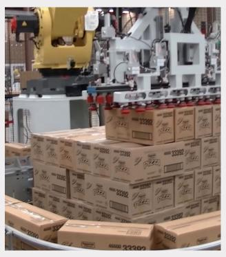
ABCO added a Fanuc robot with end-of-arm tool to pick nine meal trays and place three trays (each) into three boxes; case loading continues until there are six layers of meal trays in each case. This model robot is extremely fast and versatile with an end-of-arm tool that also picks six cases for palletizing. A single vacuum supplies the pickup for both the trays and sealed cases. This Fanuc robot is capable of carrying a maximum payload of 308 lbs., while performing a maximum reach of 112".
